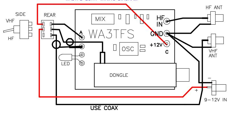
WIRE YOUR WA3TFS SDR1 CONVERTER IN THIS MANNER. RF CONNECTIONS TO AND FROM THE SWITCH SHOULD BE COAX CABLE. ANY MINIATURE COAX LIKE RG-174 IS SUITABLE. BE SURE TO CONNECT THE GROUND ON THE ANTENNA CONNECTORS TO THE GND CONNECTION ON THE CIRCUIT BOARD. POWER IS ONLY SUPPLIED WHEN THE SWITCH IS IN THE HF POSITION. POWER TO THE DONGLE IS SUPPLIED BY THE USB CONNECTION TO THE COMPUTER.
