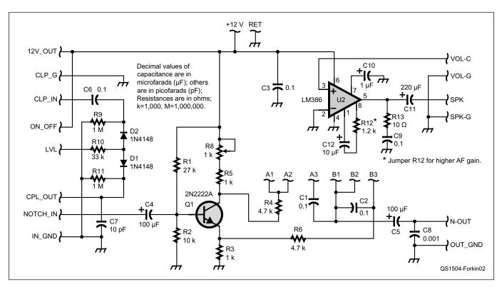
Figure 2 — Schematic diagram of the notch filter/clipper board. (Stackpole, Yageo, Vishay BC, Panasonic components from digikey.com; Kemet parts from mouser.com).
